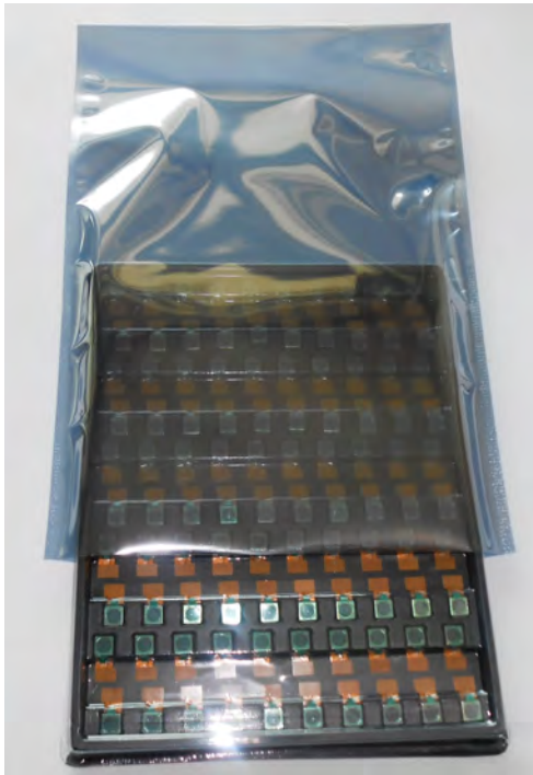
Put Tray into Anti-Static Bag
